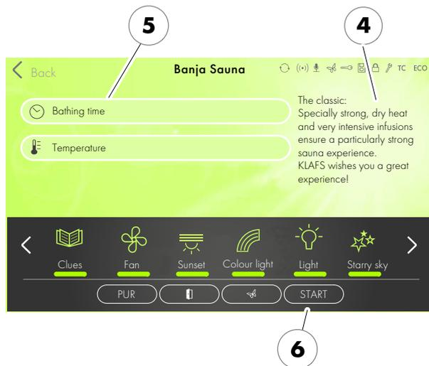
The program descriptions (4) are displayed alongside the saved bathing parameters (5) such as the temperature, humidity, intensity or bathing time.
